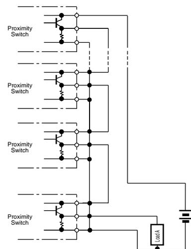
Series Connection of DC Switching Type Proximity Switches (PNP)
