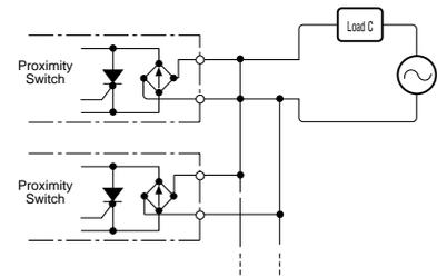
Parallel Connection of AC Switching Type Proximity Switches
