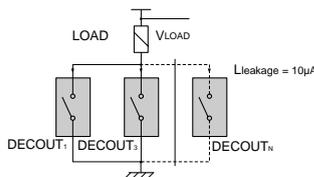
The maximum number of the sensors (n) to be connected is obtained from the formula:
